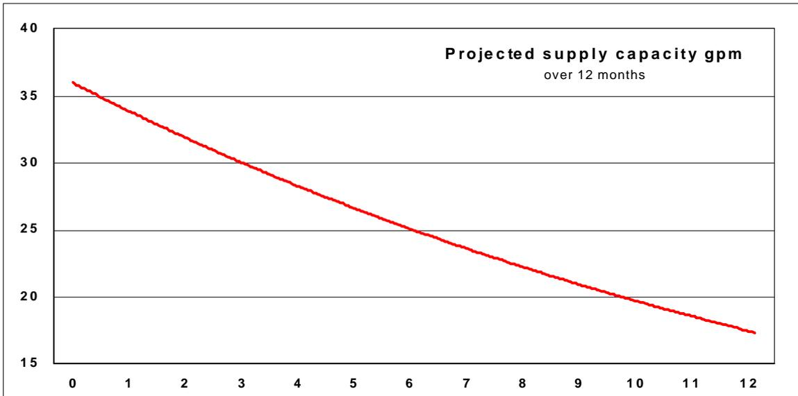
The exact cause of this progressive reduction is not exactly clear, but the most likely explanation is a progressive blocking of the supply filter by particulate matter (assuming one to be present).
