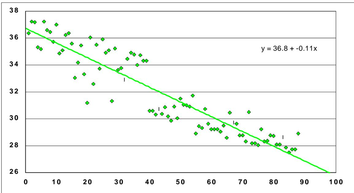
That is, the site supply is losing peak pumping/delivery capacity at the rate of about 0.11 gallon per day. On this basis, supply would drop to zero within a year.
