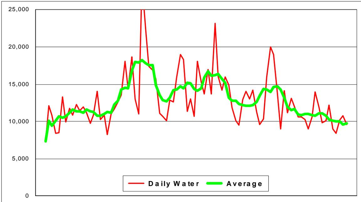
It's noted here that the daily volume is similar at the end to the beginning. Whilst a fault in the meter cannot be discounted, it seems unlikely. Looking at similar total daily volumes, it seems that early on it takes around 17 pumping hours for 12,000 gallons, whilst at the end it is around 21 hours.
