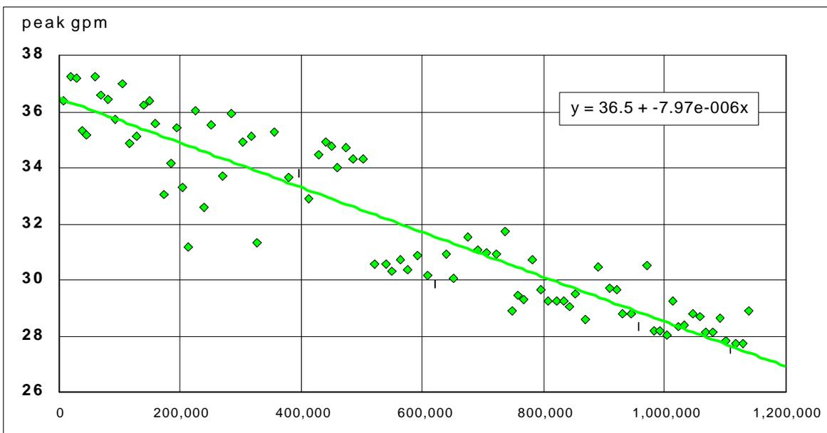
That is, the system is losing pumping capacity at the rate of 7.97 gpm per million gallons delivered i.e. 21.8% per million gallons. This averages 0.11 gpm per day. During the period measured, capacity seems to have fallen by about 23% over the period measured (from 36.5 to 28 gpm)(On this basis, supply would drop to zero within a year.
