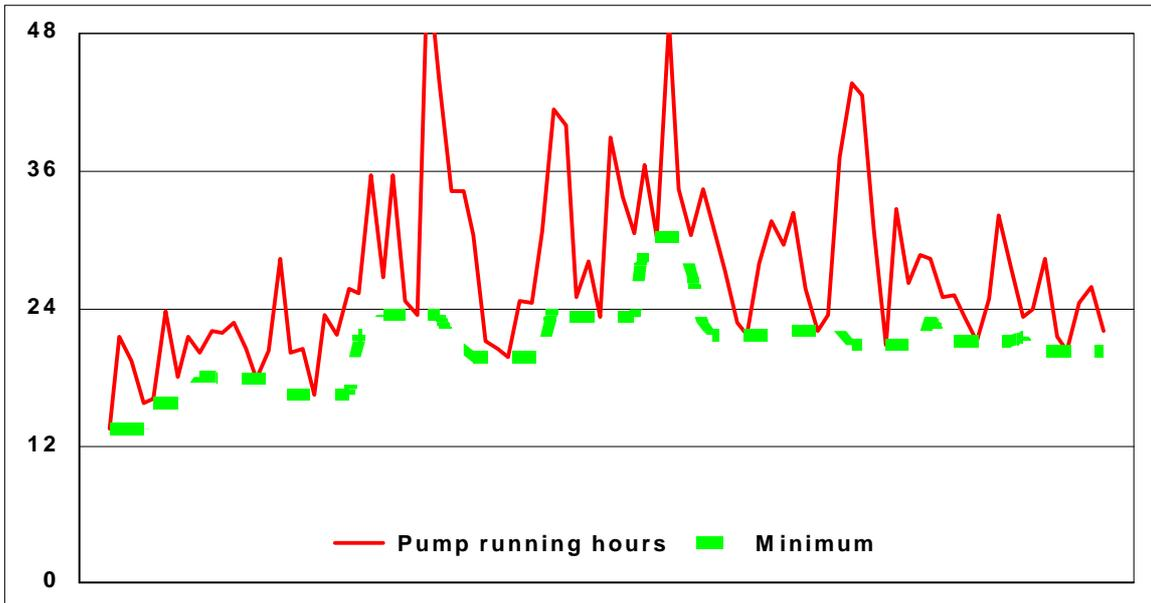
This charts shows the number of hours the pumps would need to run to supply the total volume measured, based on the pumping rate estimated by the peak rate measured. Since there are two pumps, the scale goes up to 48 (i.e. two pumps each running 24 hours). Since the actual demand varies from day to day, the Minimum line shows the least number of hours
