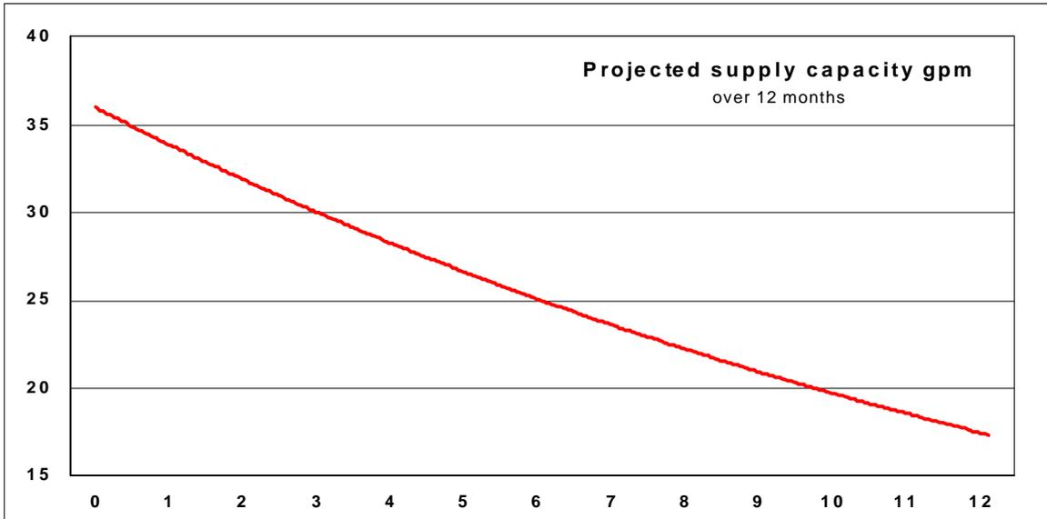
The effect of reduced peak pumping capacity would be that pumps would need to run for more hours per day.
